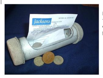
One was a mechanical system, in which gravity helped propel the cash-containing pods along wires; the other was a pneumatic system in which a blast of compressed air or suck from a vacuum had the pods in motion.
